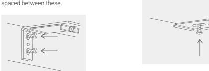
2. Attach the cassette to the bracket making sure it has caught the back lip of bracket as shown, and rotate into a horizontal position whilst keeping it tight against the bracket.
