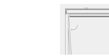
Press the adjustable sideguide into the fixed part, ensuring that the bottom bar will be free to move through it along the full drop of the blind.
