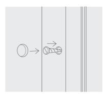
3. Insert adjustable side-guide into fixed side-guide, ensuring that the plastic bottom-bar endcap is slotted into the opening of the adjestable sideguide.
