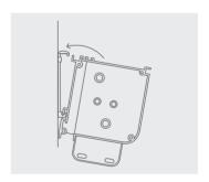
3. Slide the black plastic bracket inserts into position in each bracket, ensuring that they are fully inserted.
