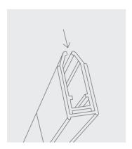
4. Slot bottom channel over the narrow part of the fixed sideguides as shown.
