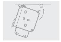
3. Slide the black plastic bracket inserts into position in each bracket, ensuring that they are fully inserted.
