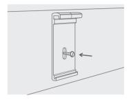
2. Set Cassette onto lower lip of bracket, as shown, and rotate into vertical position, tight against the bracket.
