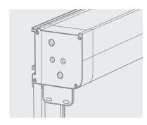
2. Once in position, screw into place at pre-drilled holes using fixings suitable for the target material.
